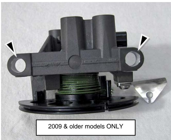
Replace throttle controller assembly in hull.
