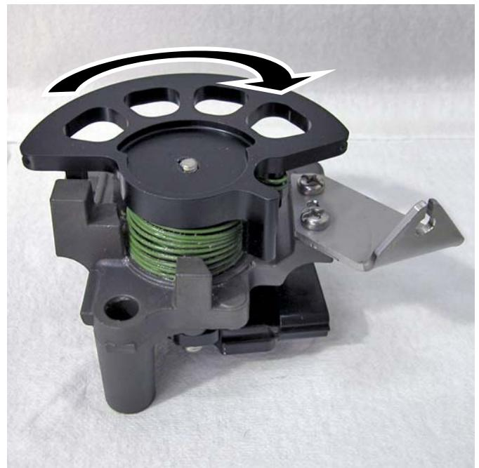
Rotate further to install throttle wheel onto throttle shaft completely. Install stock lock washer and throttle shaft nut onto throttle shaft and tighten. (see illustration #10)
